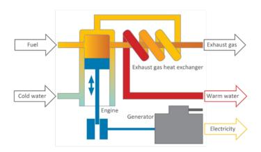
**Picture above:** A schematic representation of how a combined heat and power plant works.
